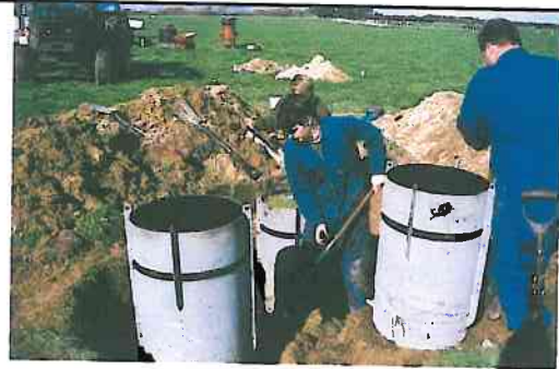
Lincoln University Dairy Farm has 60 lysimeters to measure nitrate leaching from free-draining soils on North Block.
